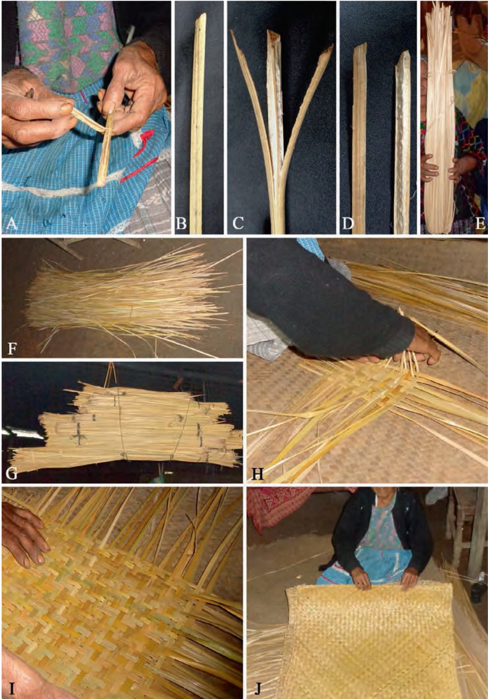
Fig. 5. Production of mats ' petates ' with tulle; A-E – selection and preparation of stem barks, F–G – stem barks of different dimensions, H–I – interlacing process of the stems, J – finished mats (Photo. E. M6)
