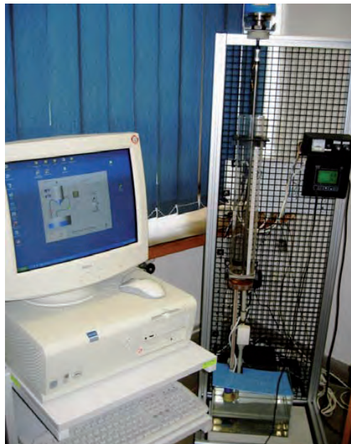
Fig. 9. Model of level tank control with industrial controller in connecting with PC computer
