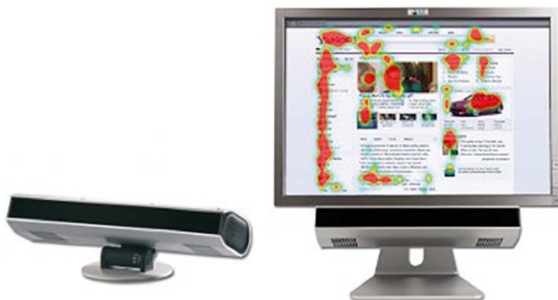
Ryc. 5.8. Systemy RED ( Remote Eyetracking Device )
