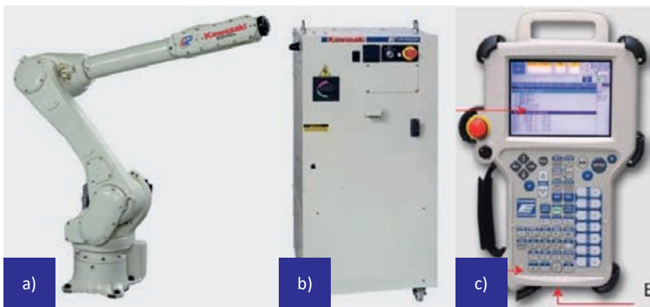
Fig. 6. The Robot Kawasaki RS006L type installed at the Institute of Technology of the Pedagogical University of Cracow (a- robot arm; b-CPU; c-Teachpendant)
