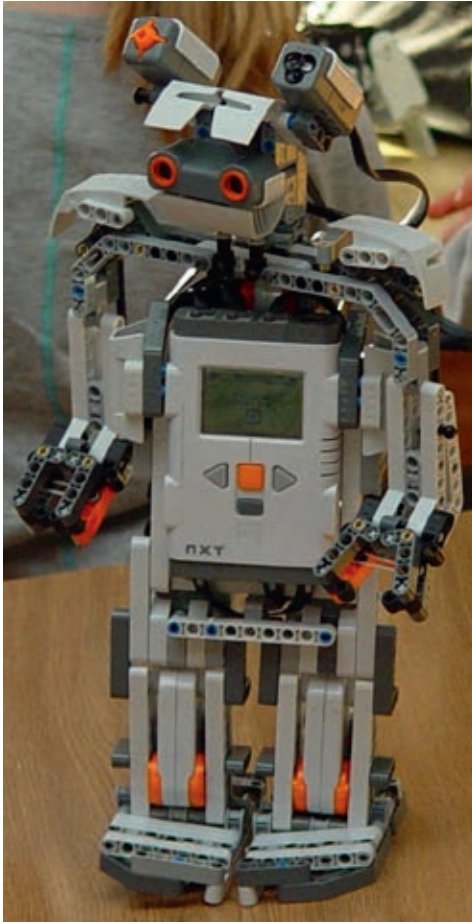
Fig. 2. Humanoid robot made of Lego bricks
