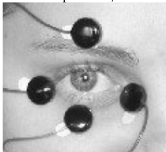
Figure 19: Method of connecting electrodes used in measuring changes in eye positioning by using the electric method (Augustyniak 2001, p. 69).
