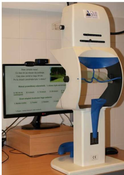
Figure 31: The High Speed Eyetracker SMI 1250 Hz in Neurodidactics Laboratory at the Pedagogical University of Cracow, Institute of Physics.
